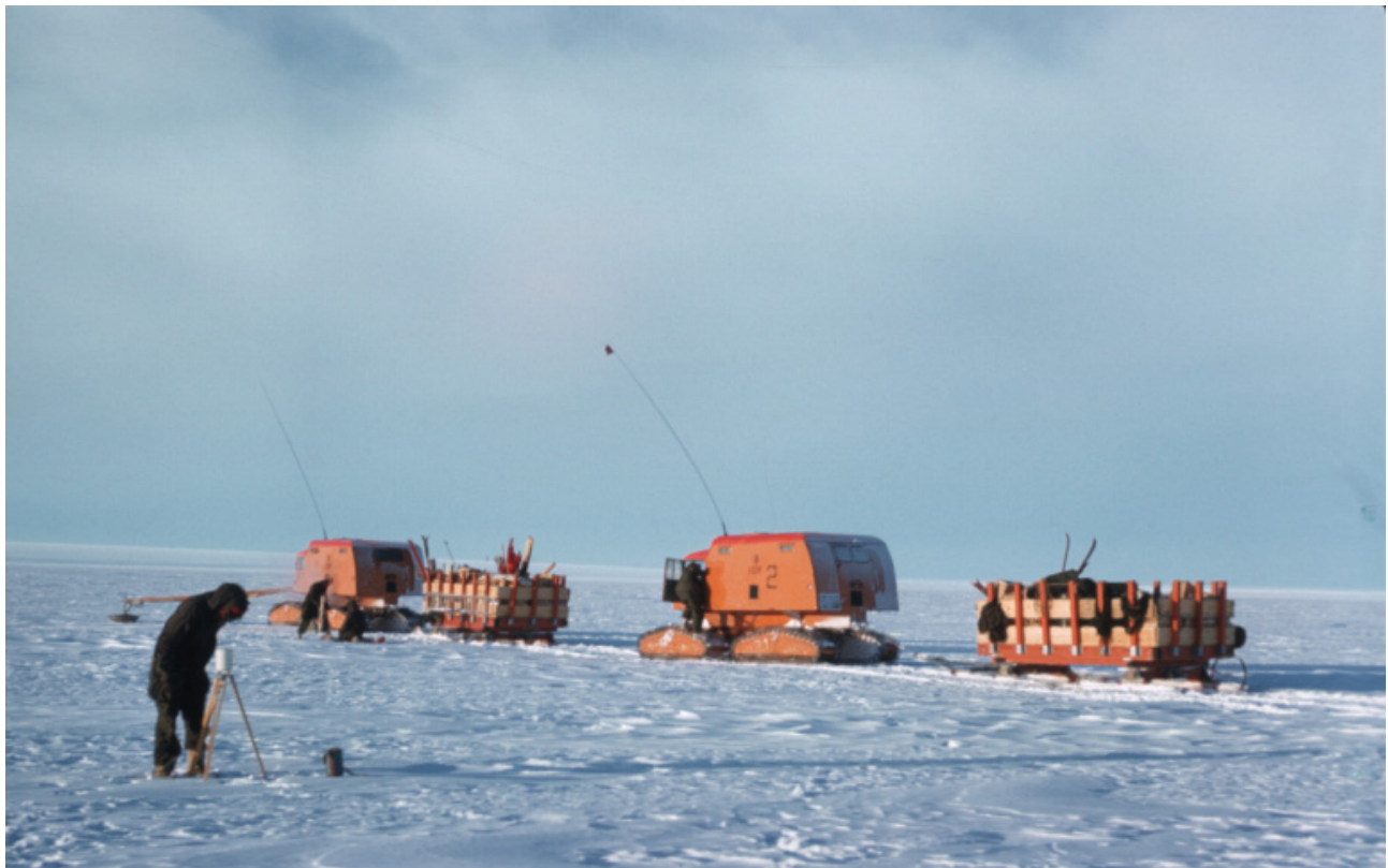
Fig. 1. Traverse at intermediate station. Behrendt reading magnetometer at left. Walker and Aughenbaugh making snow hardness measurement left background. Thiel on track of Sno-Cat after making a gravity measurement. Crevasse detector visible on leading vehicle.
